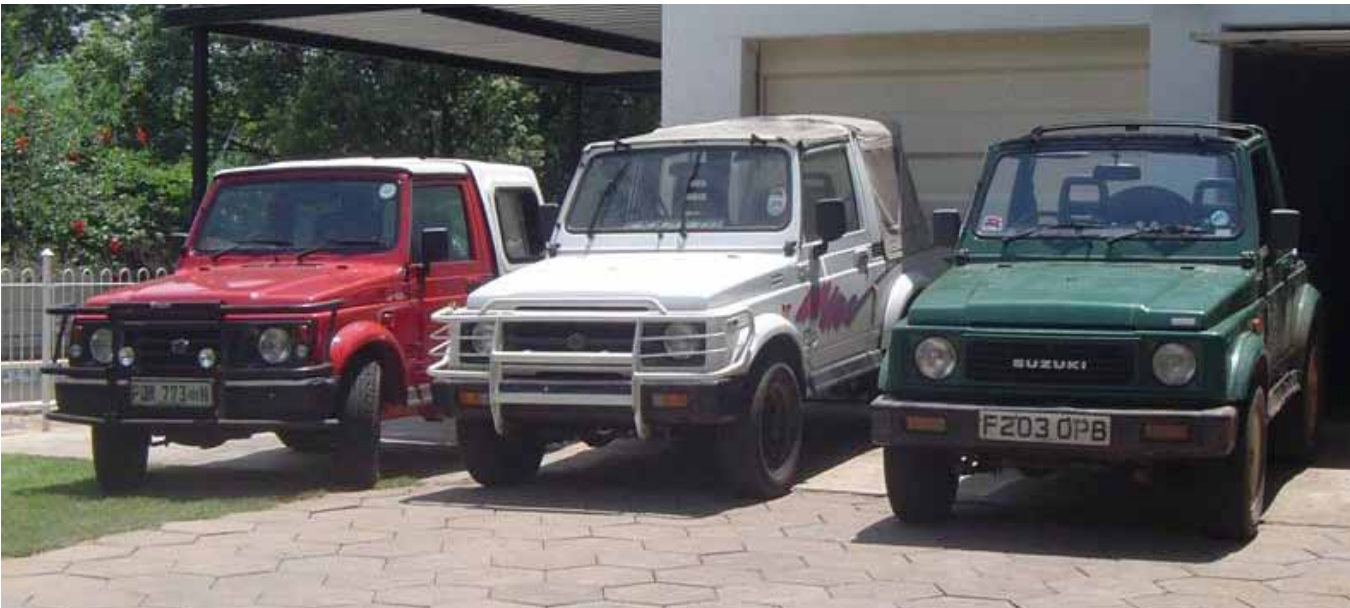
Here one can see the difference in Samurai 1300 grilles from my personal 2004 Suzuki-collection: Green = 1988 ; white = 1993; red = 1997 (the '96 onwards are usually referred to as "coily", due to coil spring suspension)
