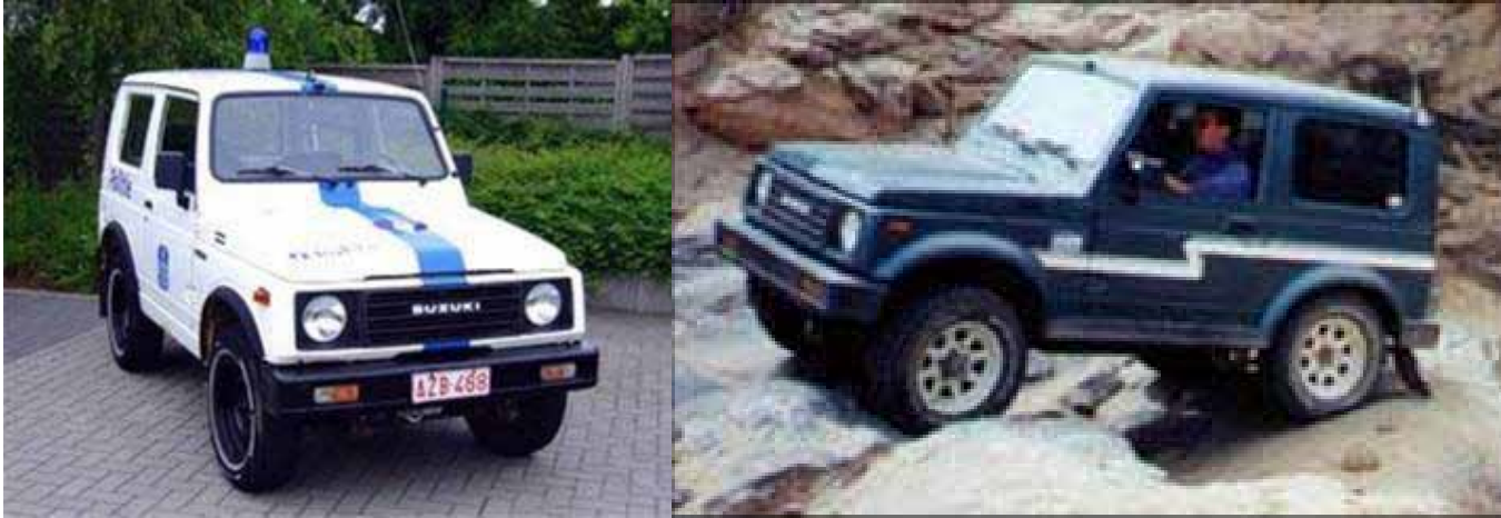
SJ413 SW (1986 version, note the smaller plastic strips around the wheel arches on the white SJ VS. the later, 1988 blue one's wider wheel arch extensions )
